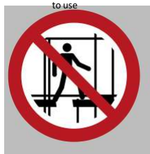
P025 Using the incomplete scaffolding prohibited
