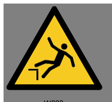
W008 Warning danger of falling
