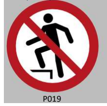
P019 Climbing prohibited
