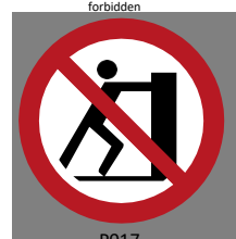
P017 Pushing prohibited
