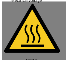
W017 warning of hot surface
