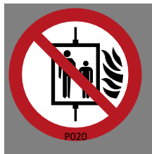
P020 Elevator not in case of fire to use
