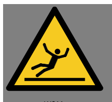
W011 Warning Danger of slipping
